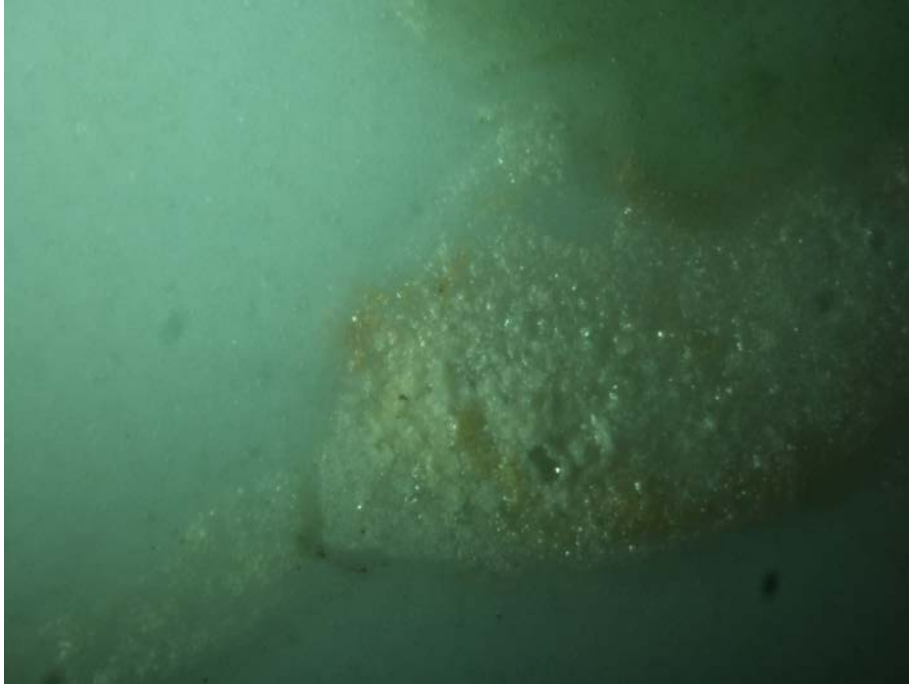
Four Seasons Ware 1093°, 2 hr. Showing Bubbling/Dissipation of Enamel Decoration.
