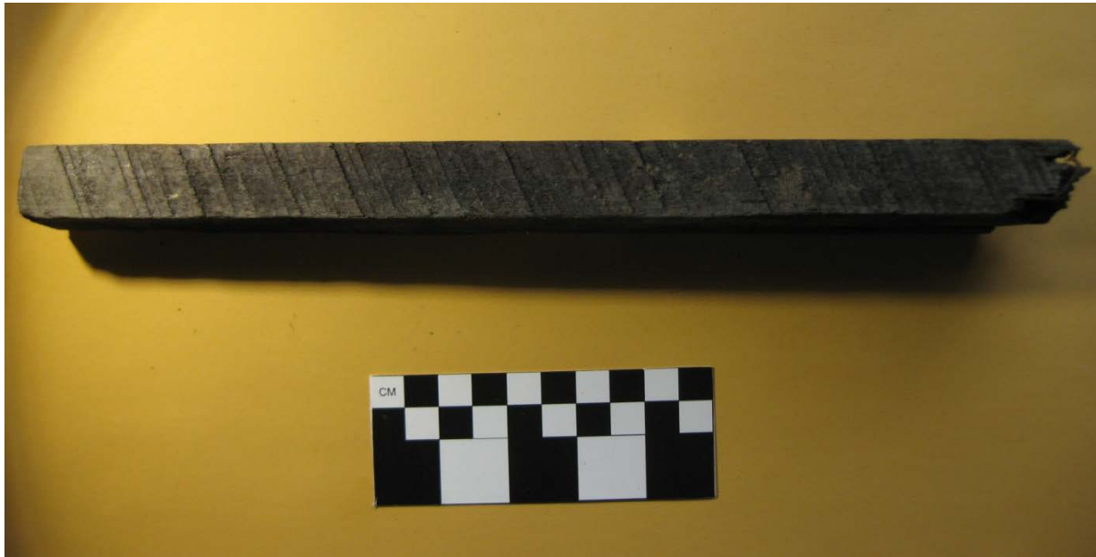
Figure 1. Timber from 86-36/2-94 with circular saw tool marks
